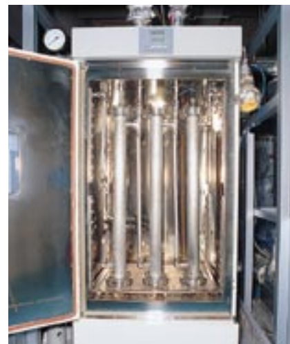
*TOX-FREE*, a system which removes dioxin from exhaust gas
