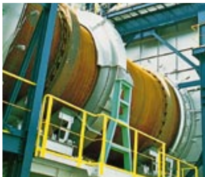
Slagging rotary kiln which incinerates and melts industrial waste
