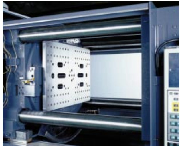
図3 反転装置 Mold rotary device
