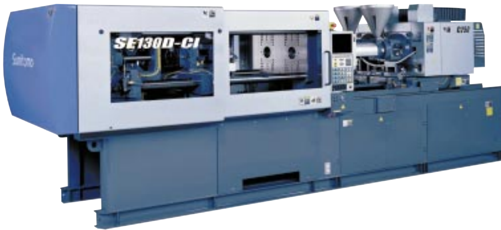
図1 全電動 2 材成形機 Fully electric double-shot injection molding machine
