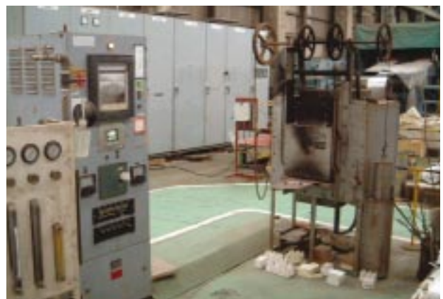
図7 炉内雰囲気調整機能付き電気炉 Electric oven with atmosphere controller
