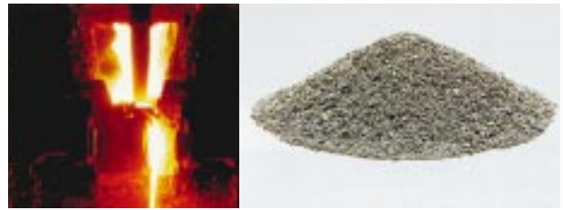
図5 出滓滓口と水砕スラグ Slag tap and slag crushed water
