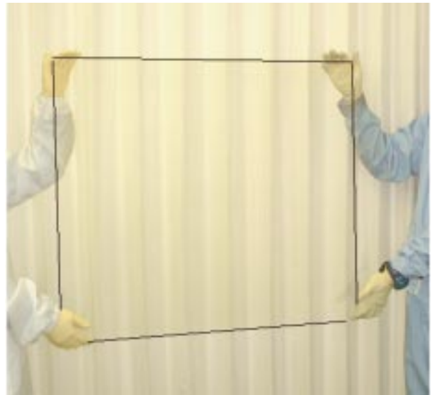
図4 RPD法による920 x 730基板へのGZO成膜 GZO film on 970 x 730 substrate coated by RPD method
