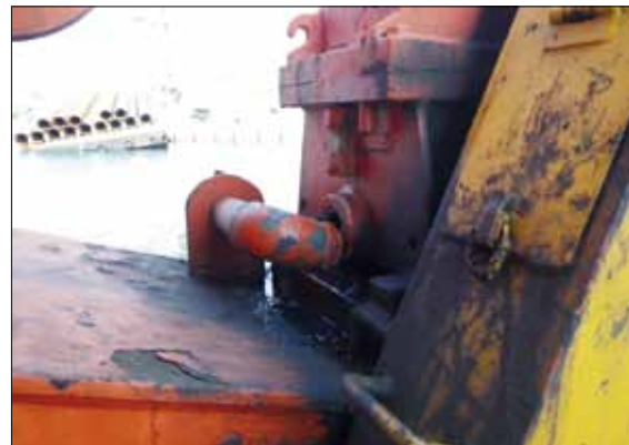
図4 減速機破損 Broken reducer gear system
