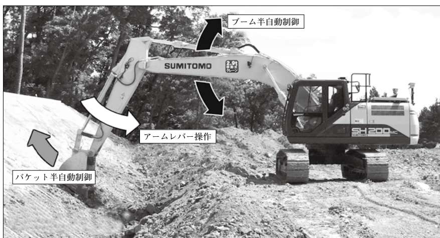
図6 MC仕様の半自動制御 SH200-7 MC semi-automatic control
