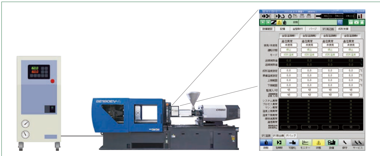
図1 温調機管理画面 Management screen of mold temperature controller
