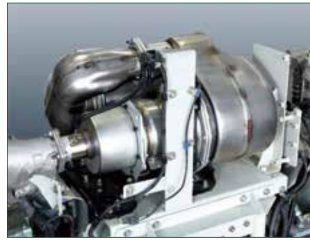
図5 後処理装置 Exhaust gas after treatment device
