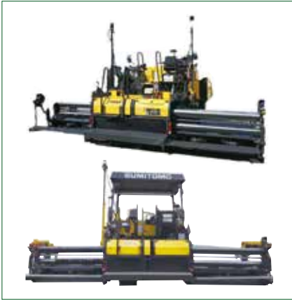
図3 3D-MC機器装着状態 3D-MC device mounting state
