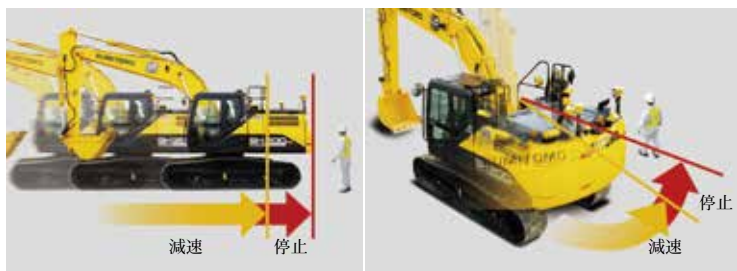
図3 走行・旋回時の減速・停止制御のイメージ Image of control for reducing speed and stop on moving and turning
