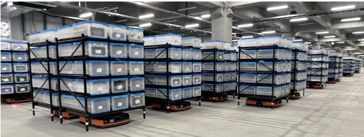
図3 AGVとGTP用保管棚
